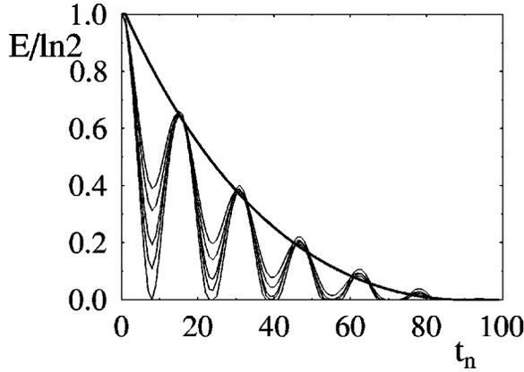
FIG. 4. Dependence of entanglement of formation on time for several randomly chosen maximally entangled pure states. The unitary dynamics  $U = \exp(i\alpha\bar{H})$  is governed by the parameter  $\alpha$ . Here  $\epsilon = 0.01$  in  $\vec{p}^{(2)}$ , and  $\alpha = 0.1$  (narrow lines). Reference bold line represents the case of no unitary dynamics ( $\alpha = 0$ ), for which the dynamics of entanglement does not depend on the initial state.
